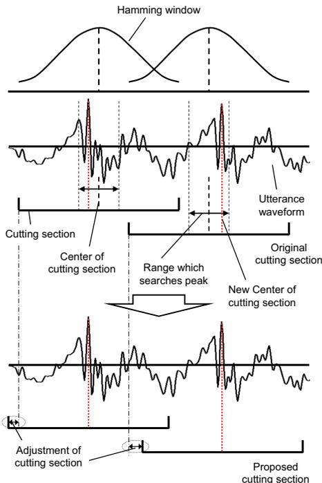
Figure 2: How to synchronize the splitting section.
