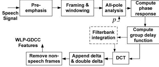
Figure 3: All-pole group delay-based countermeasures extraction stages.
