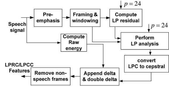
Figure 4: Block diagram showing various steps to extract linear prediction cepstral coefficients (LPCC) and linear prediction residual cepstral coefficients (LPRC) by performing LP analysis of actual speech signal and residual signal, respectively.
